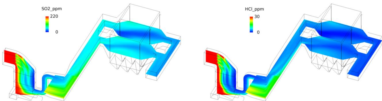
Fig. 2. CFD predictions of (left)  $\text{SO}_2$  and (right) HCl species concentration a DSI hydrated lime injection on a 200-MWe unit.
