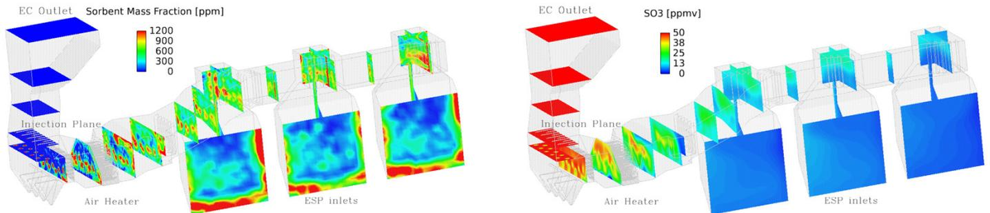
Fig. 1. CFD predictions of hydrate lime particle concentration (up) and  $\text{SO}_3$  species concentration (low) for a DSI application on a 500-MWe unit flue gas duct. CFD Domain starting from economizer outlet to ESP inlet.
